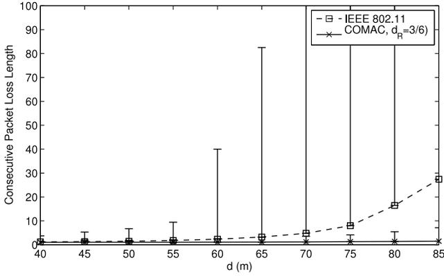
Fig. 8. Mean and maximum lengths of consecutive packet losses at the controller vs.  $d$  using both COMAC and IEEE 802.11 MAC
