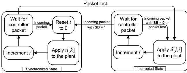
Fig. 3. Operation of the actuator node.
