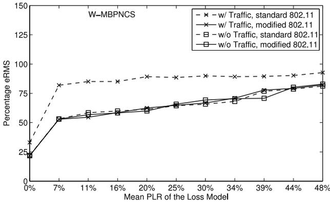
Fig. 6. Controller performance of W-MBPNCs over IEEE 802.11 under bursts of packet loss, using standard and modified MAC, with and without ambient wireless traffic
