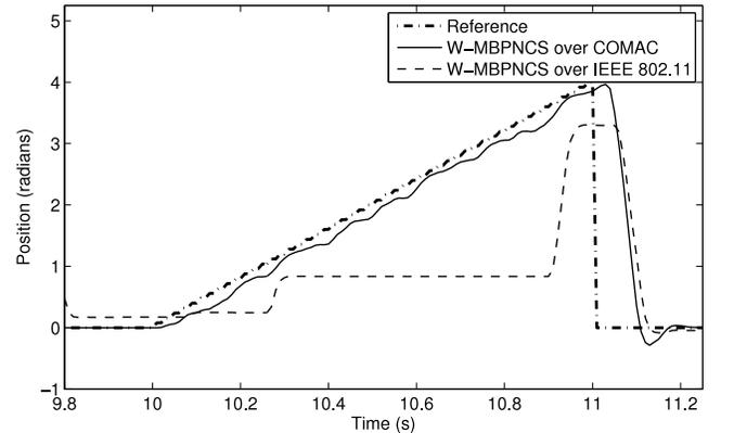
Fig. 11. Sawtooth reference vs. plant output using COMAC under Rayleigh Fading
