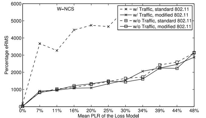
Fig. 5. Controller performance of the conventional W-NCS over IEEE 802.11 under bursts of packet loss, using standard and modified MAC, with and without ambient wireless traffic
