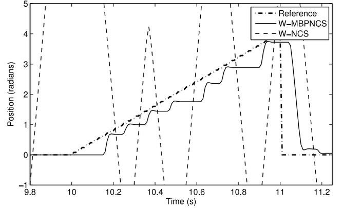
Fig. 7. Sawtooth reference vs. plant output using IEEE 802.11 MAC under bursts of packet loss
