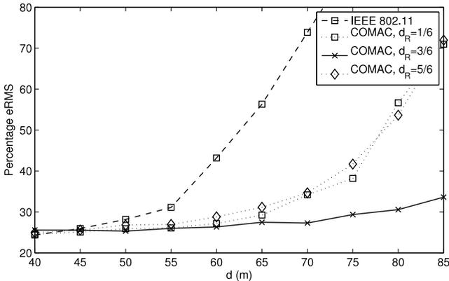
Fig. 9. Controller performance of W-MBPNCs over COMAC under Rayleigh fading vs.  $d$
