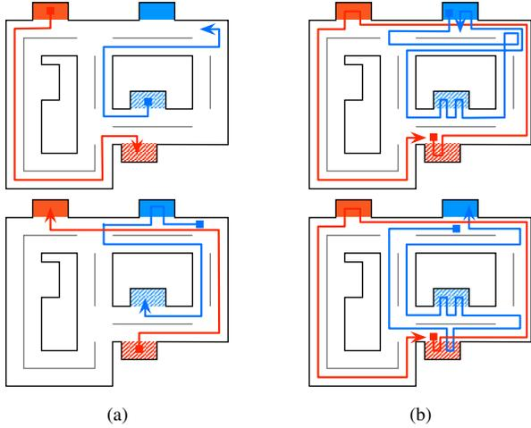
Fig. 5: Simulated team trajectories for the two case studies. (a) and (b) correspond to the cases where the weights are within the ranges  $\{1 \dots 5\}$  and  $\{1 \dots 20\}$ , respectively. Robot 1 and robot 2 travel between red and blue task locations respectively. Regions filled with a solid color are data gathering locations and regions with a diagonal pattern are upload locations.
