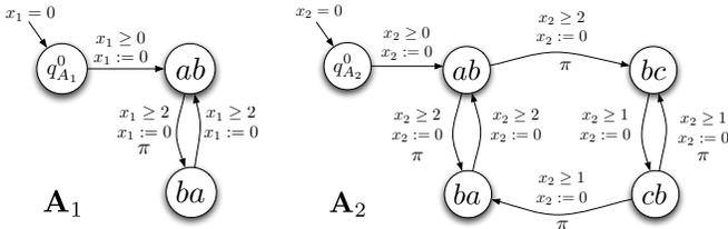
Fig. 2:  $A_1$  and  $A_2$  of each robot, corresponding to  $D_1$  and  $D_2$  shown in Fig. 1c and Fig. 1d, respectively. The equations next to each arrow represents the clock constraint and the clock-reset associated with the transition.
