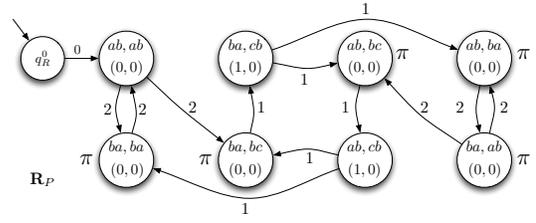
Fig. 3: The finite state region automaton capturing the joint behavior of two robots in 9 states. In the circle representing a state  $\{q, r\}$ , the first line is  $q$  and the second line is  $r$ .
